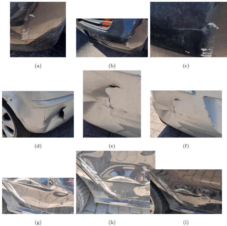
Fig. 1. Example of damage similarities. Triplets (a)–(b)–(c), (d)–(e)–(f), and (g)–(h)–(i) are real matches of the same damages. Each row shows an example type of damage: scratch , crack , and dent , respectively.
