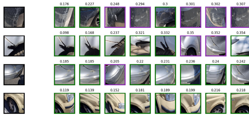
Fig. 4. Sample queries and matching images in the public test set. The leftmost images are query images, followed by the highest similarity matches. Images framed in green are correct reidentifications, whereas those in purple indicate errors. The similarity score is also shown above each image. Even in cases of error, the model identifies images that are very similar to the query one.
